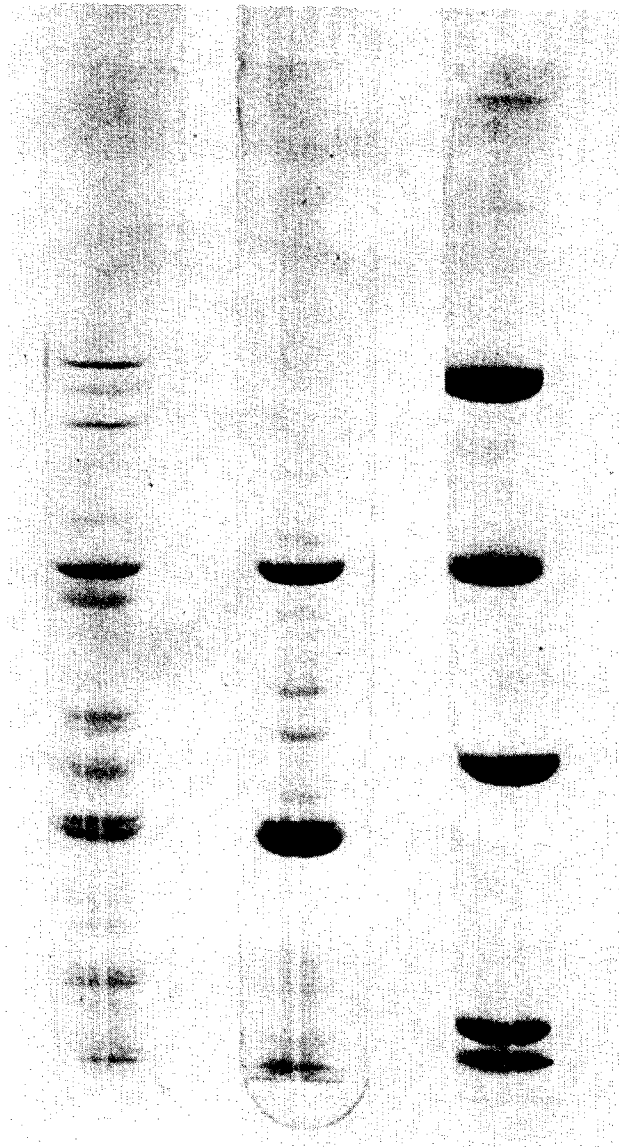
Fig. 3. SDS acylamide gel electrophoresis. From left to right: Sample II, Sample I, and standards. The standards applied were BSA, ovalbumin, carbonic anhydrase, \beta -lactoglobulin, and cytochrome C with 68,000, 43,000, 32,000, 18,000 and 12,000 mol. wt., respectively. To obtain samples I and II, microsomal estrogen binders were partially purified on Sephadex G100 followed by DEAE cellulose chromatography, which yielded 2 EBP peaks, peaks I and II. These were rechromatographed, separately, on Sephadex G100, thereby providing for Samples I and II, respectively.
